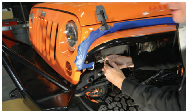
14. Unbolt and remove the Crusher Flare.
