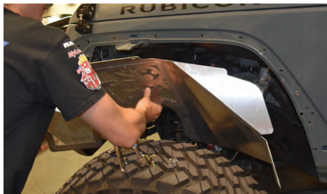
16. Carefully insert the Inner Fender piece into the wheel opening. Make sure the correct piece is being used on each side.
