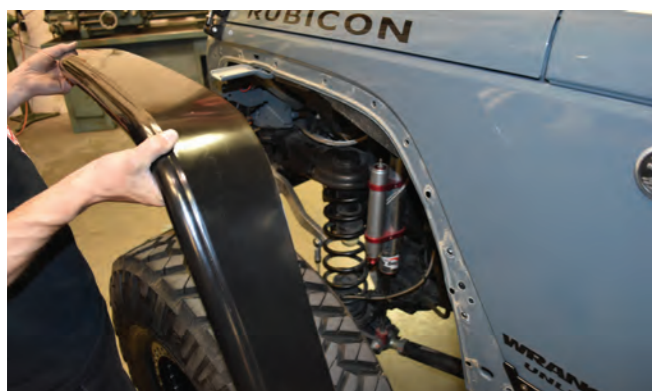
15. Remove the Crusher Flare Lower Sub-Frame Bracket from the rearward side of the wheel opening.
