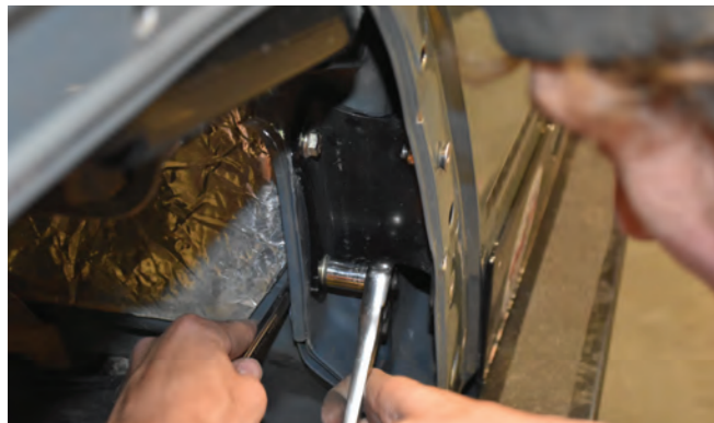
16. Carefully insert the Inner Fender piece into the wheel opening. Make sure the correct piece is being used on each side.
